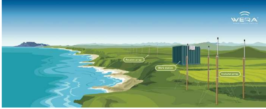
Figure 2: Sketch of WERA Ocean Remote Sensing System.
